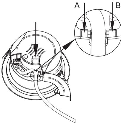
5. Press the clamp into the holes "A" and "B" to fix the cord.
