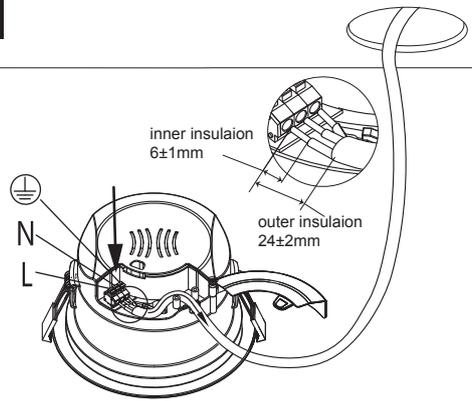
4. Individually connect the Live wire, Neutral wire and Ground wire of AC input wire to L/N and ground terminal of downlight and put the cord between the 2 pillars.
