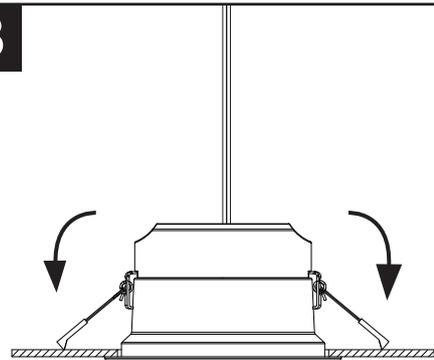
8. Release the spring and make sure the downlight is firmly in place.
