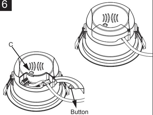
6. Rotate the cover back until the button fits into the hole "C" and make sure the cover could not open without pressing the button.
