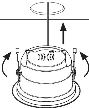
7. Push the spring up and place downlight in the ceiling.
